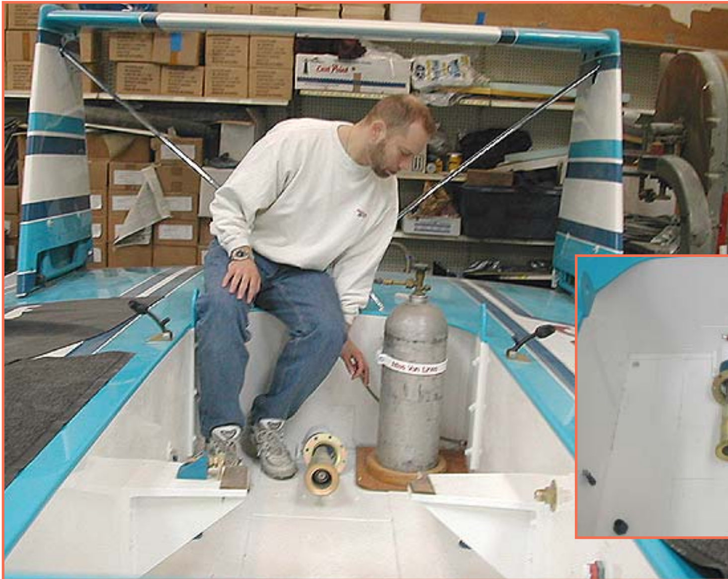
Rear engine compartment view shows shaft-log and coupler. Atlas crewman Jeff Stubbers checks the nitrous bottle mount. The two water overboard fittings in the bottom can be seen in the photo below.
